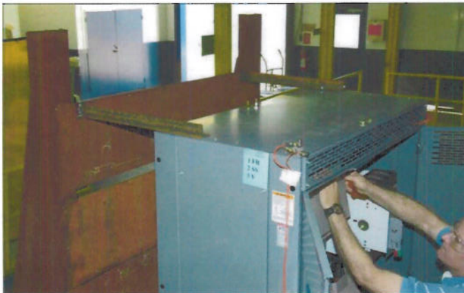
Photo 3 - Addition of top lateral restraints for high level test demand.
