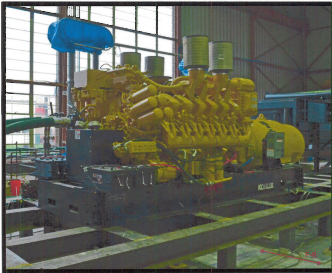
The 1250 kW REOZDC generator skid is anchored to the test fixture with 8-7/8" diameter A490 bolts (4 per side).
