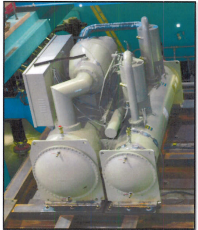
RTHD D2G3G3 mounted on 'VMC' elastomeric pad anchored to the test fixture, an extension of the table, with 12-3/4" diameter Grade 8 bolts.
