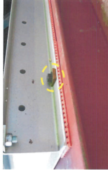
Figure 9. Bolted connection and elastomeric pad between the UUT1 skid and adapter frame
