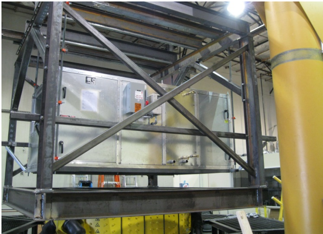
UUT4, mounted to DCL shake table interface frame, instrumented and ready for test.
