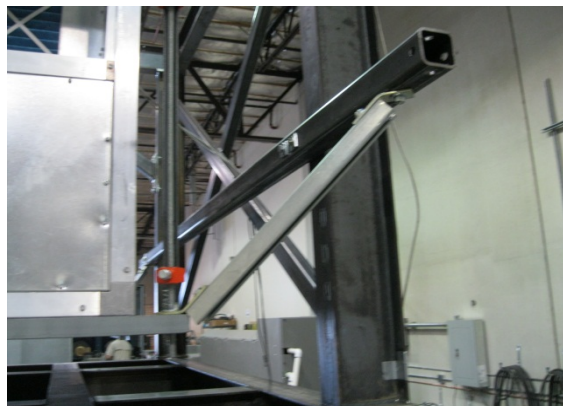
UUT4 close-up of mounting hardware (brackets, lateral bracing and threaded rod with stiffener).
