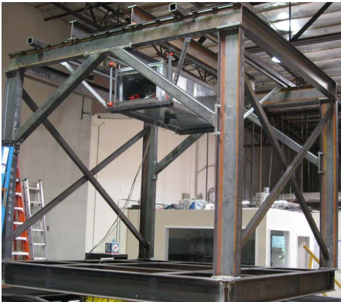
UUT3, mounted to DCL steel shake table interface frame, instrumented and ready for test.
