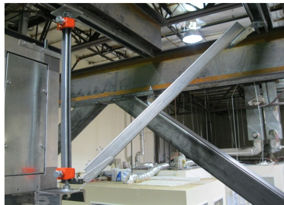
UUT3 close-up of mounting hardware (brackets, lateral bracing and threaded rod with stiffener).
