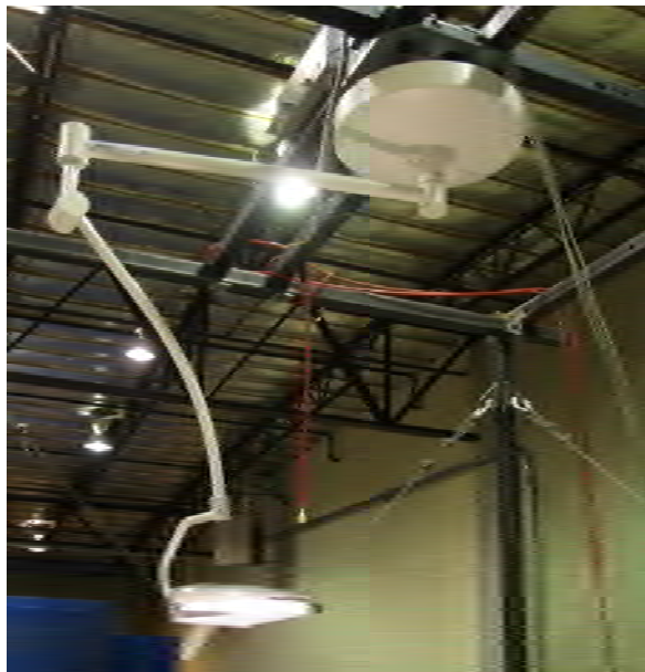
UUT3a, mounted to test frame, instrumented and ready for test.
