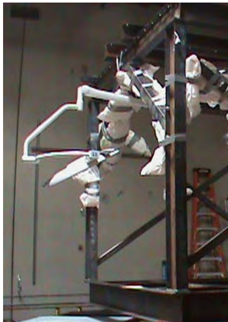
UUT7, mounted to test frame, instrumented and ready for test.
