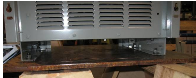
Charger bolted to plate using four 3/8"-16 bolts with standard washers (one bolt in each corner)
