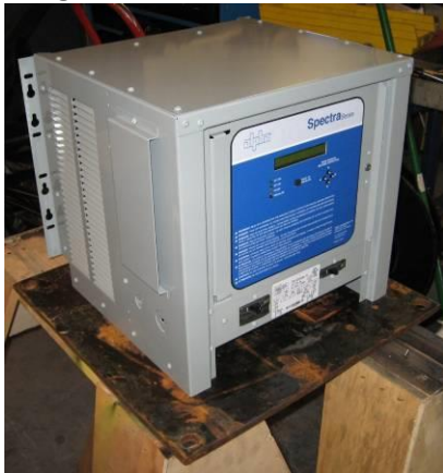
Charger bolted to plate using four 3/8"-16 bolts with standard washers (one bolt in each corner)
