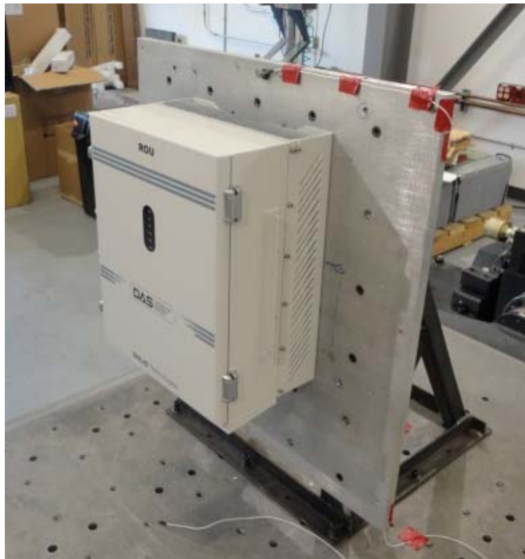
UUT 3 on Rigid Wall Mount
