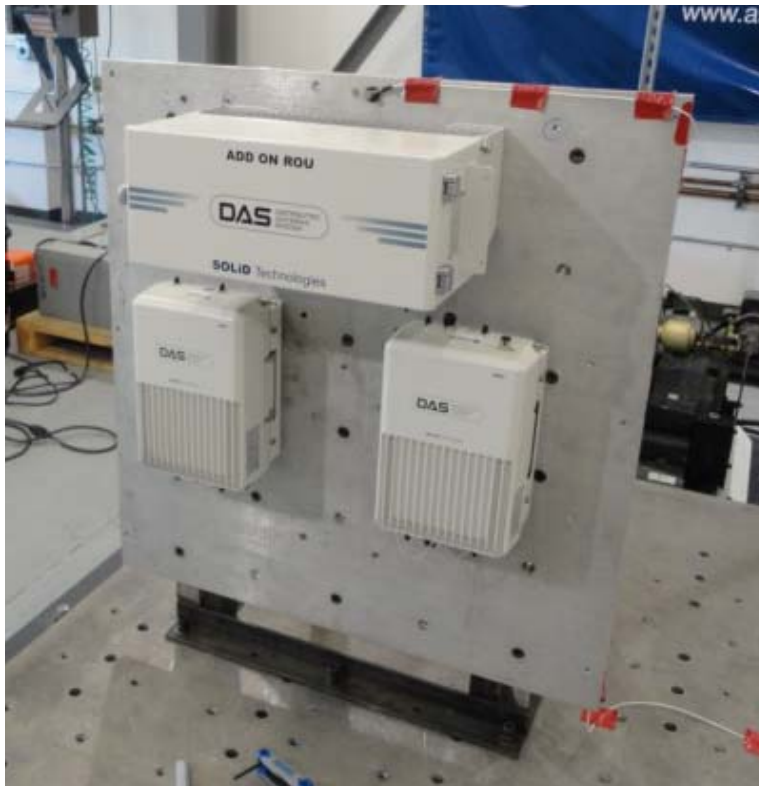
UUT 4 on Rigid Wall Mount
