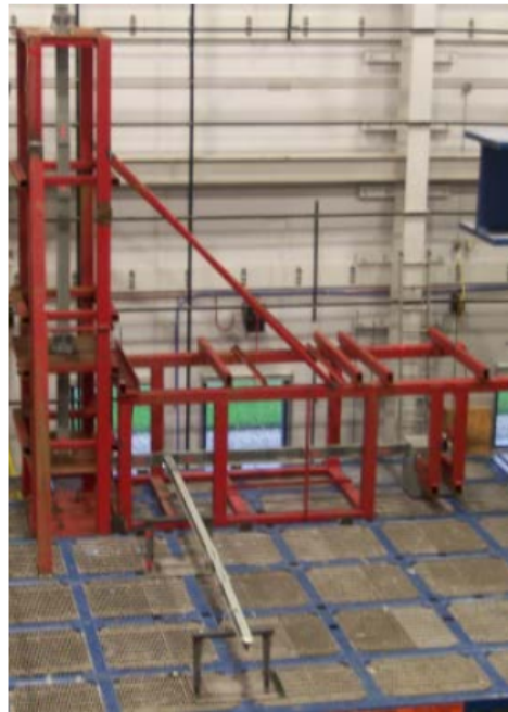
Figure 2-6: South view of UUT3 mounted on support frame attached to shake table
