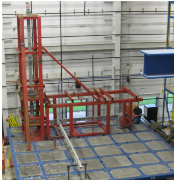
Figure 2-7: South view UUT4 mounted on support frame attached to shake table
