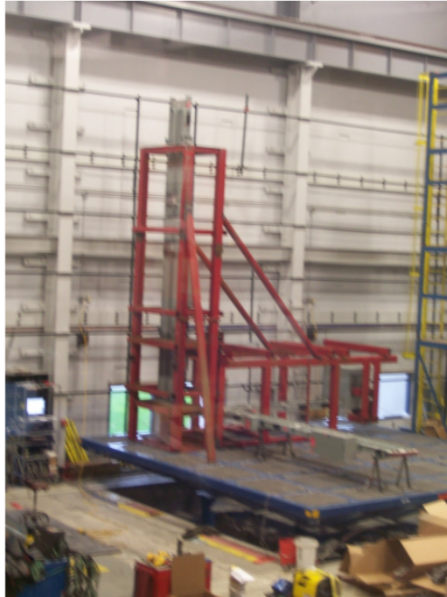
Figure 2-4: Southwest view of UUT1 mounted on support frame attached to shake table
