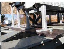
24 grade 8 1/4"-20 bolts were used to hold the rack to the table (2 bolts per foot, 8 feet per stand, 3 stands).
