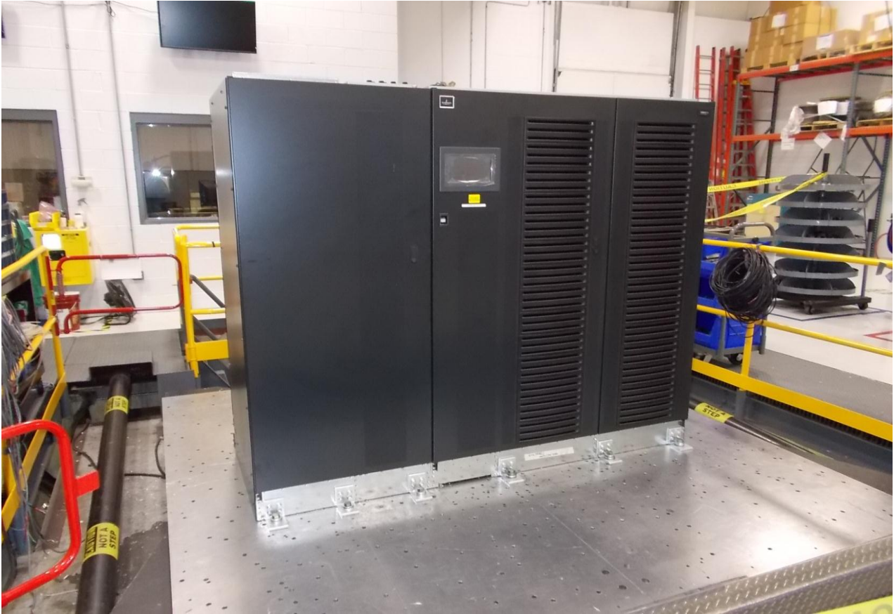
Figure 2: NX 600kVA UPS Attachment Method: rigid-mount - (13) 3/4"dia bolts to table, angle brackets by Liebert A_{FLX-H} = 3.63 ; A_{RIG-H} = 2.72 ; Unit maintained structural integrity and functionality after the ICC-ES AC-156 test.
