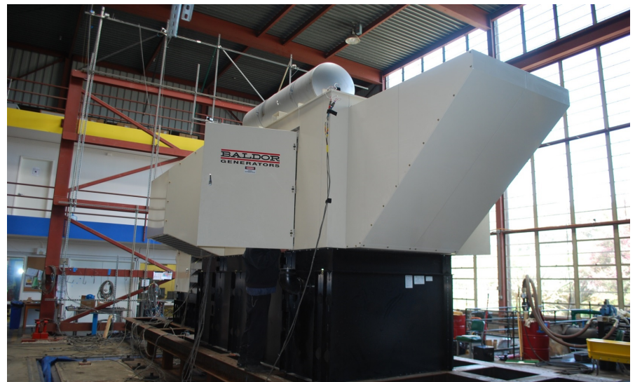
UUTs 3A & 3B (Same Unit Tested With and Without Water) Sub-Base Fuel Tank is Mounted Directly to the Fixture Using (12) 3/4" Diameter ASTM
