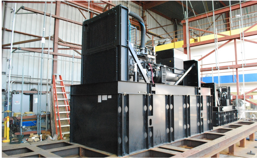
UUTs 4A & 4B (Same Unit Tested With and Without Water) Sub-Base Fuel Tank is Mounted Directly to the Fixture Using (12) 3/4" Diameter ASTM A490 Bolts.
