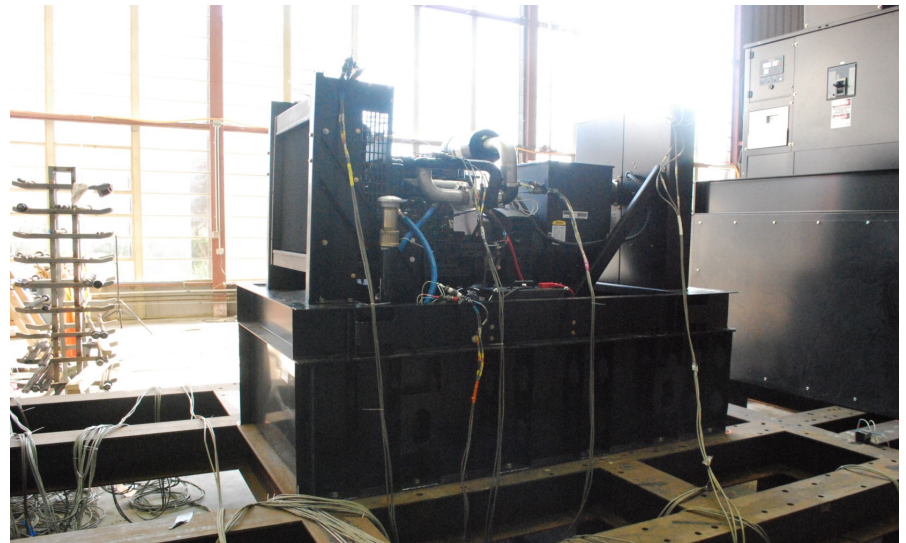
UUTs 2A & 2B (Same Unit Tested With and Without Water) Sub-Base Fuel Tank is Mounted Directly to the Fixture Using (12) 3/4" Diameter ASTM A490 Bolts.
