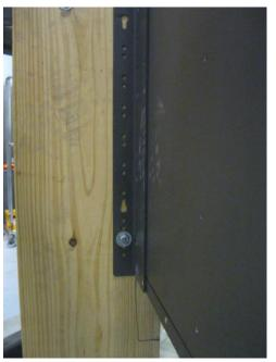
Mounted to test fixture using (4) 3/8" x 1" long lag bolts. Test fixture mounted to table using (16) 1/2" Grade 8 bolts. Unit maintained structural integrity and remained functional per manufacturer requirement.
