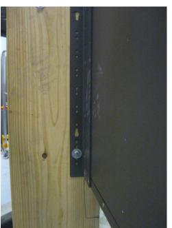
Mounted to test fixture using (6) 3/8" x 1" long lag bolts. Test fixture mounted to table using (16)  $\frac{1}{2}$ " Grade 8 bolts. Unit maintained structural integrity and remained functional per manufacturer requirement. Contents were included in testing per operating conditions.
