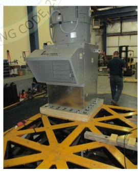
UUT was mounted to 24" roof curb using (16) 5/16" thread cutting screws. Roof curb was mounted to a 6" wood base using (24) 5/8" lag bolts (ASTM Grade A307-A). Unit maintained structural integrity and remained functional per manufacturer requirement after shake table test. Contents were included in testing per operating conditions.
