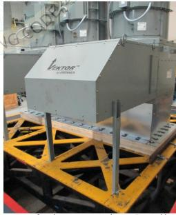
UUT was mounted to 24" roof curb using (36) 5/16" thread cutting screws. Roof curb was mounted to a 6" wood base using (40) 5/8" lag bolts (ASTM Grade A307-A). Each weatherhood used two vertical supports which bear on the table but were not positively attached to it. Unit maintained structural integrity and remained functional per manufacturer requirement after shake table test. Contents were included in testing per operating conditions.
