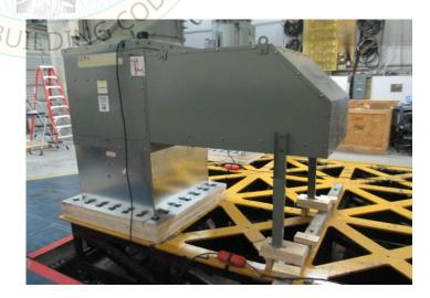
UUT was mounted to 24" roof curb using (16) 5/16" thread cutting screws. Roof curb was mounted to a 6" wood base using (24) 5/8" lag bolts (ASTM Grade A307-A). The weatherhood used two vertical supports which bear on the 6" wood base but were not positively attached to it. Unit maintained structural integrity and remained functional per manufacturer requirement after shake table test. Contents were included in testing per operating conditions.
