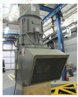
UUT was mounted to 24" roof curb using (12) 5/16" thread cutting screws. Roof curb was mounted to a 6" wood base using (20) 5/8" lag bolts (ASTM Grade A307-A). Unit maintained structural integrity and remained functional per manufacturer requirement after shake table test. Contents were included in testing per operating conditions.
