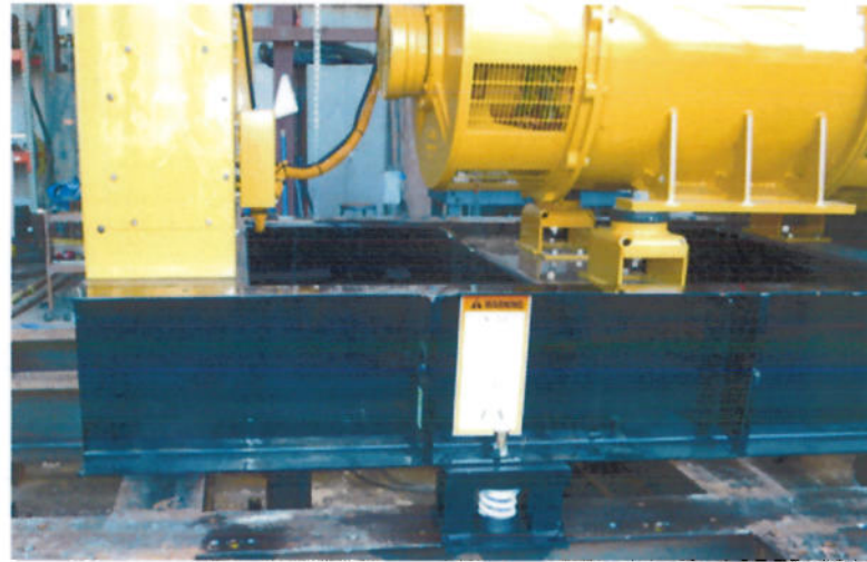
UUT 1B, No tank, on VMC MSSH-1E Isolators
