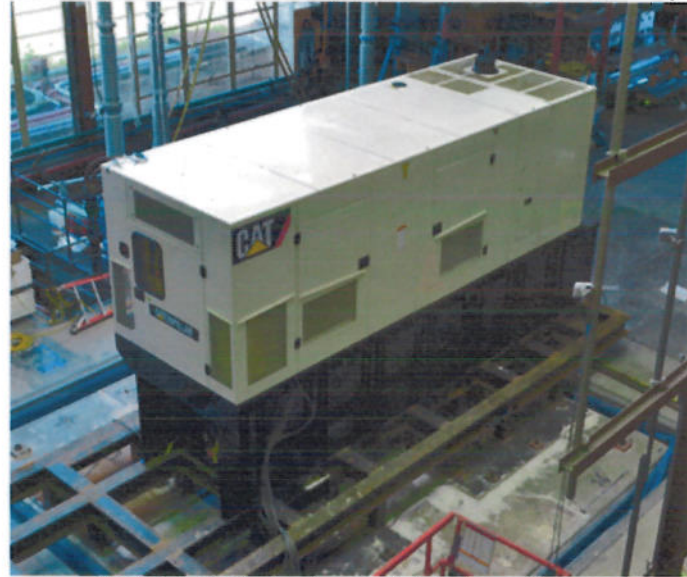
UUT 2A & 2B, Enclosed, on tank, bolted to table
