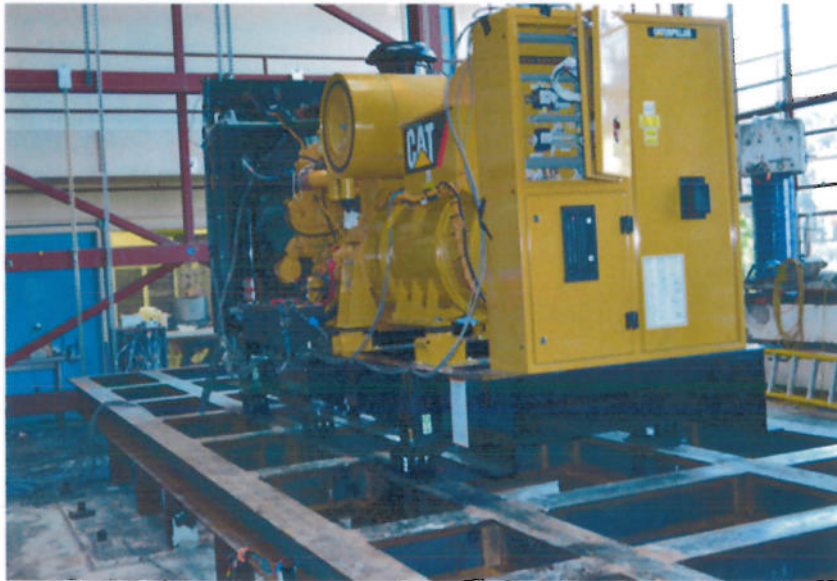
UUT 1B, No tank, on VMC MSSH-1E Isolators
