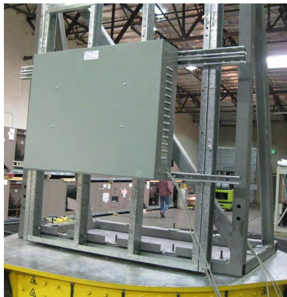
UUT4, wall-mounted to shake table interface frame.
