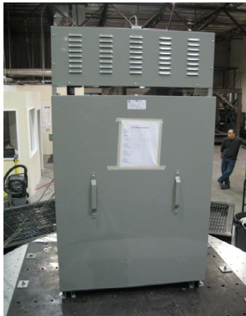
UUT5, floor-mounted to shake table interface plate.
