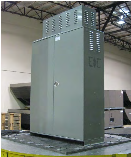
UUT1, floor-mounted to shake table interface plate.
