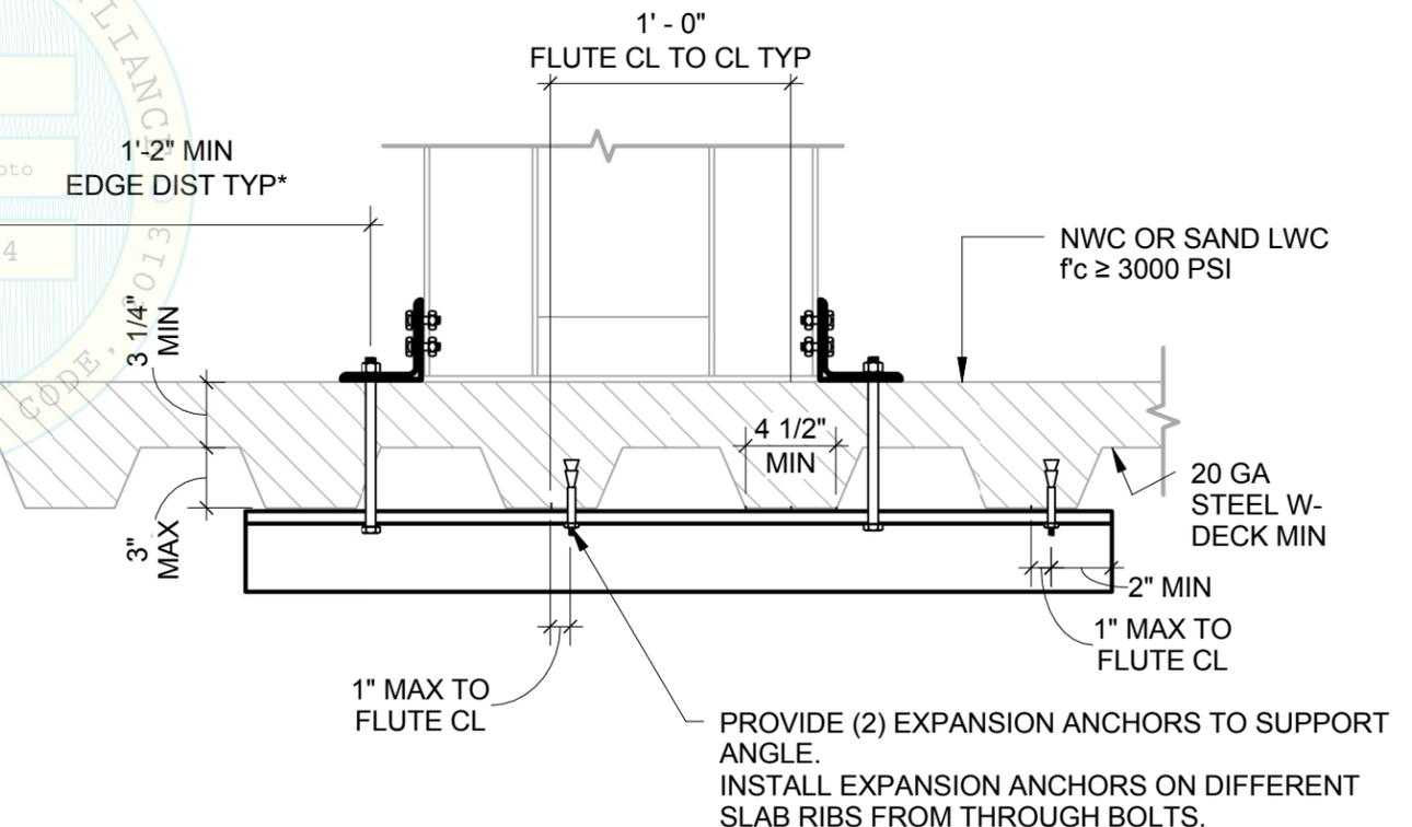
\*PROVIDE 8" MINIMUM DISTANCE TO EDGE OF SLAB, OPENINGS OR OTHER ATTACHMENTS
