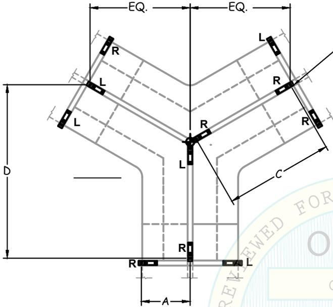
INDICATES SEISMIC ATTACHMENT:
