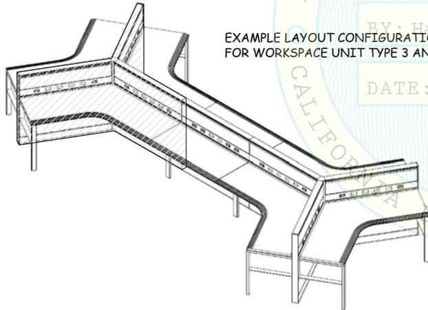
EXAMPLE LAYOUT CONFIGURATIONS FOR WORKSPACE UNIT TYPE 1 AND 3.
