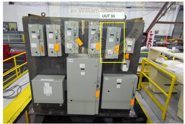
UUT 31 was mounted to a rigid frame using (3) 1/4" bolts. The steel frame was welded to the shake table.
