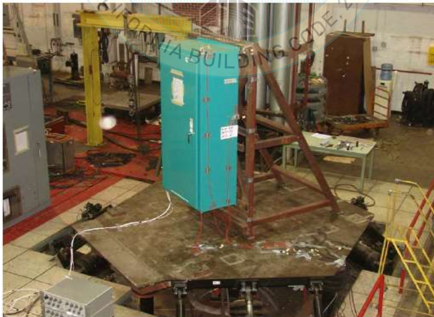
Figure 2 OPC 600A Cabinet mounted on Tri-axial Table
