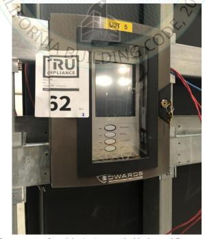
UUT 62 was rigid mounted to a wall fixture using four (4) 3/16" ungraded bolts and flat washers. Unit maintained structural integrity and remained functional per manufacturer requirement after shake table test. Contents were included in testing per operating conditions.
