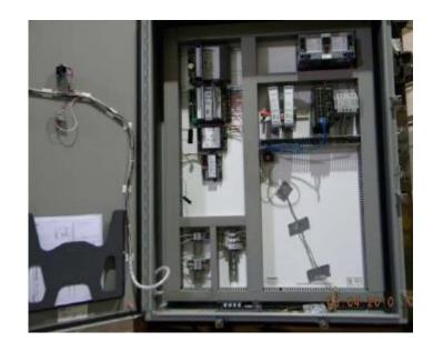
Rigid wall mounted to wall fixture with (4) 5/16" cap screws. Unit maintained structural integrity and remained functional per manufacturer requirement. Contents were included in testing per operating conditions.
