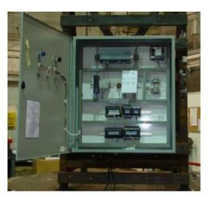
Rigid wall mounted to wall fixture with (4) 5/16" cap screws. Unit maintained structural integrity and remained functional per manufacturer requirement after shake table test. Contents were included in testing per operating conditions.
