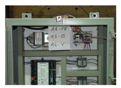
Rigid wall mounted to wall fixture with (4) 3/8" cap screws. Unit maintained structural integrity and remained functional per manufacturer requirement after shake table test. Contents were included in testing per operating conditions.
