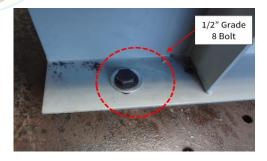
Base mounted-rigid using four (4) 1/2" -13 SAE Grade 8 bolts with lock washers and flat washers. Unit maintained structural integrity and remained functional per manufacturer requirement after shake table test. Contents were included in testing per operating conditions.
