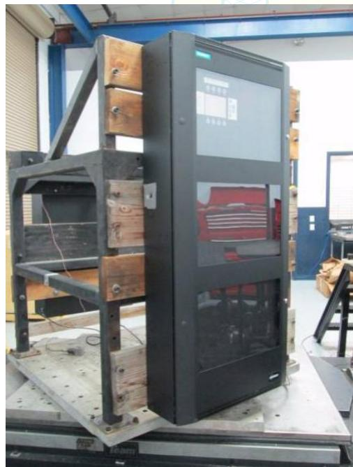
UUT was rigid wall mounted using (6) 5/16" Grade 8 bolts. Unit maintained structural integrity and remained operational per manufacturer requirement following shake table test. All contents were included in the unit per operating conditions.
