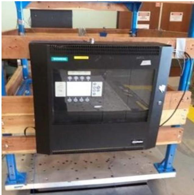
UUT was rigid wall mounted using (4) 3/8" x 1.25" lag screws.
