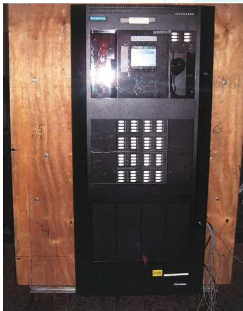
UUT was rigid wall mounted using (6) Grade 2 or less #14x1" Type A bolts.
