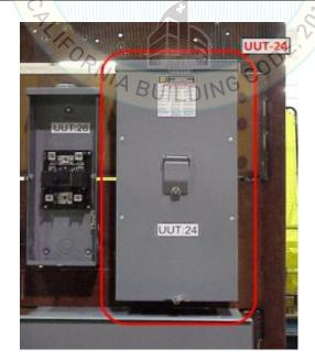
UUT was rigid wall mounted using (4) 1/4" grade 5 bolts and flat washers torqued to 7 ft-lbs. Unit maintained structural integrity and remained functional per manufacturer requirement after shake table test. Contents were included in testing per operating conditions.
