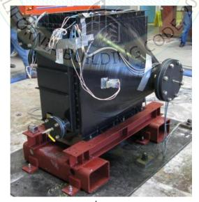
UUT2b was mounted to I-beams with eight (8) 1/2" A307 bolts<sup>1</sup>. The GENSET rail was mounted to the shake table with eight (8)1/2" A307 bolts.
