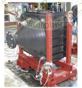
UUT2a was mounted to I-beams with twelve (12) 1/2" A307 bolts<sup>1</sup>. The I-beams were mounted to the GENSET rail with eight (8) 1/2" A307 bolts and the GENSET rail was mounted to the shake table with eight (8)1/2" A307 bolts.
