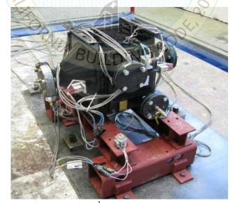
UUT1b was mounted to I-beams with six (6) 1/2" A307 bolts<sup>1</sup>. The GENSET rail was mounted to the shake table with eight (8)1/2" A307 bolts.
