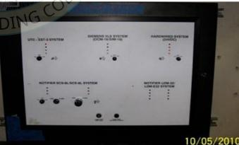
UUT2 was wall mounted - rigid using four (4) 1/4"-20 bolts into spring nuts in surface mounted strut channel. Unit maintained structural integrity and remained functional per manufacturer requirement after shake table test. Contents were included in testing per operating conditions.
