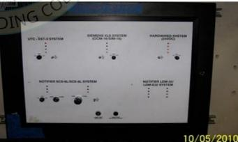
UUT1 was wall mounted - rigid using four (4) 1/4"-20 bolts into spring nuts in surface mounted strut channel. Unit maintained structural integrity and remained functional per manufacturer requirement after shake table test. Contents were included in testing per operating conditions.
