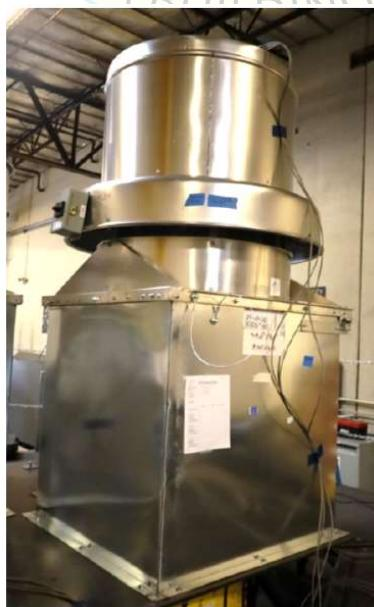
All units were filled with contents and maintained structural integrity and functionality after AC-156 test.
