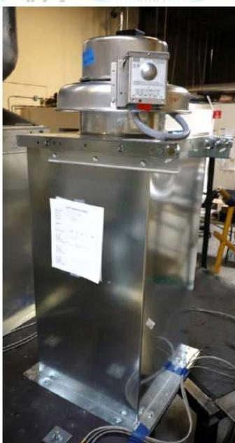
All units were filled with contents and maintained structural integrity and functionality after AC-156 test.
