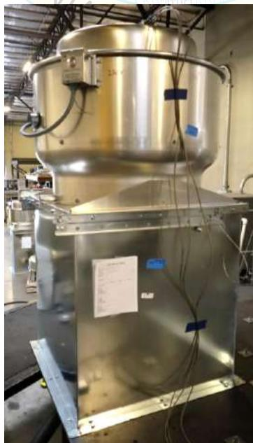
All units were filled with contents and maintained structural integrity and functionality after AC-156 test.
