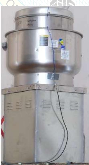
All units were filled with contents and maintained structural integrity and functionality after AC-156 test.
