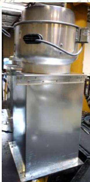
All units were filled with contents and maintained structural integrity and functionality after AC-156 test.
