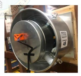
Rigid wall mounted to wall bracket on rigid wall fixture. Bracket mounted to wall with (12) 5/16" grade 8 bolts with washer. Unit mounted to bracket with (16) 1/4" Tek screws.
