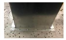
Base mounted rigid on 17.5" x 17.5" x 42" curb. Curb mounted to table with sixteen (16) 5/16" Grade 8 bolts with washers. UUT curb mounted to top of curb with sixteen (24) 1/4" Tek screws.
