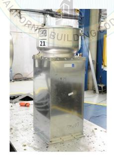
Base mounted rigid on 42" Roof Curb using (16) 5/16" self-tapping srews to attach fan to curb & (12) 5/16" Grade 8 bolts to attach curb to curb mount.
