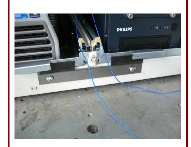
Figure 10: Detail of Sliding Shelf Retaining Clip
