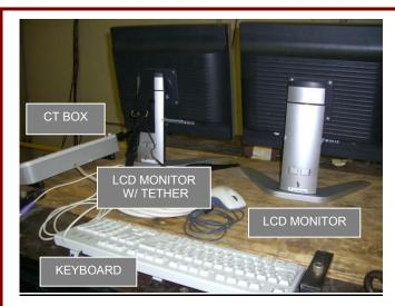
(1)-LCD MONITOR TETHERED WITH A SINGLE QUAKE HOLD! UNIVERSAL FLAT SCREEN SAFETY STRAP. ALL OTHER COMPONENTS PLACED UNANCHORED ON TEST PLATE.
