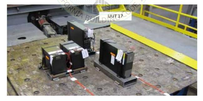
UUT17 was base mounted - rigid with Eaton Seismic Mounting Kit (SMKITA) using four (4) 1/2" Grade 8 bolts and washers. Unit maintained structural integrity and remained functional per manufacturer requirement after shake table test. Contents were included in testing per operating conditions.
