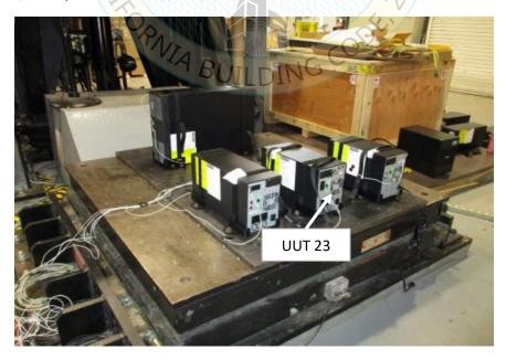
UUT23 was base mounted - rigid with Eaton Seismic Mounting Kit (SMKITA) using four (4) 1/2" Grade 8 bolts and washers. Unit maintained structural integrity and remained functional per manufacturer requirement after shake table test. Contents were included in testing per operating conditions.
