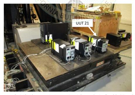
UUT21 was base mounted - rigid with Eaton Seismic Mounting Kit (SMKITA) using four (4) 1/2" Grade 8 bolts and washers. Unit maintained structural integrity and remained functional per manufacturer requirement after shake table test. Contents were included in testing per operating conditions.
