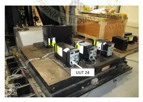
UUT24 was base mounted - rigid with Eaton Seismic Mounting Kit (SMKITA) using four (4) 1/2" Grade 8 bolts and washers. Unit maintained structural integrity and remained functional per manufacturer requirement after shake table test. Contents were included in testing per operating conditions.
