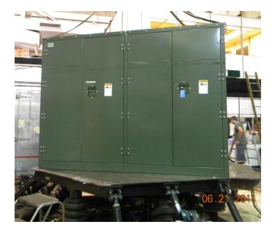
Unit mounted to table using (8) 5/8"-11 Hex Head Bolts.
