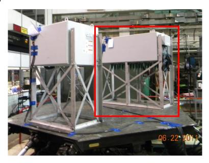
Unit mounted to table using (4) 5/8"-11 Hex Head Bolts.
