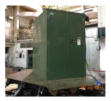
Unit mounted to table using (8) 5/8"-11 Hex Head Bolts.
