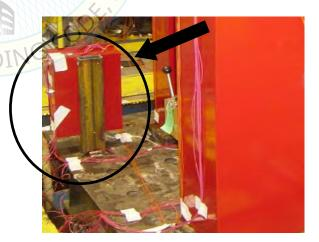
The UUT was bolted to a Wyle-fabricated test fixture using three 5/16-inch Grade 5 bolts. The test fixture was welded to the seismic test table so that the horizontal axes of the UUT were colinear with the horizontal axes of the test table.
