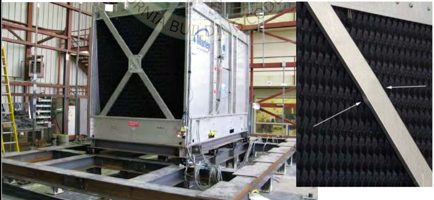
All units were filled with contents and maintained structural integrity and functionality after AC-156 test.
