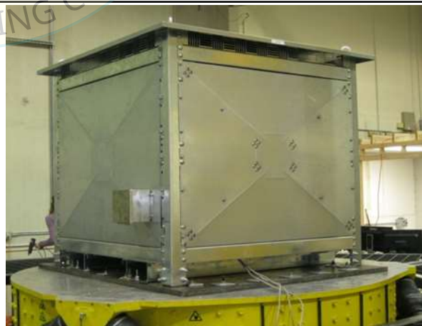
UUT4A mounted to shake table and ready for test.
