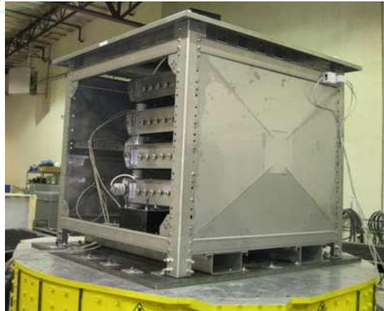
Unit mounted on shake table and ready for test (side panel removed for photograph).
