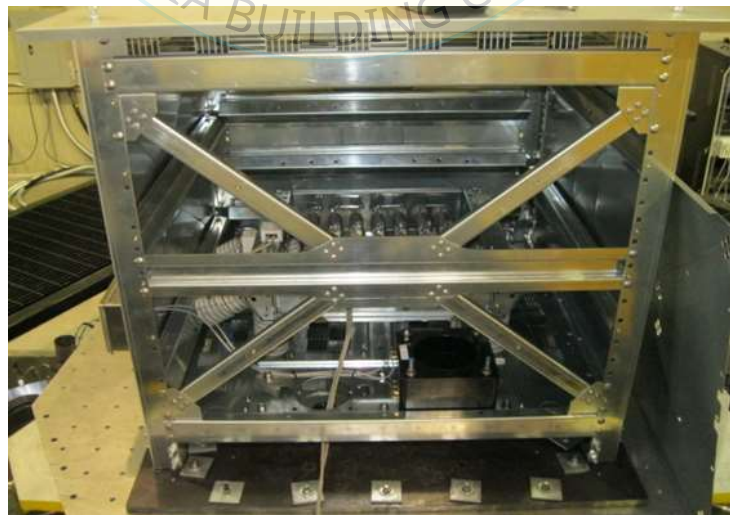
UUT3A mounted to shake table and ready for test. Side panel removed for viewing of interior.
