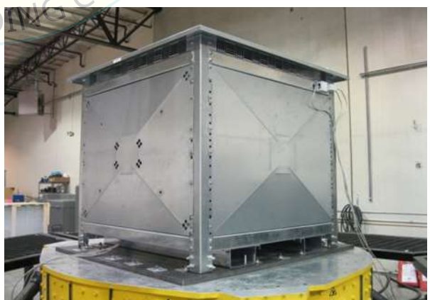
Unit mounted on shake table and ready for test.
