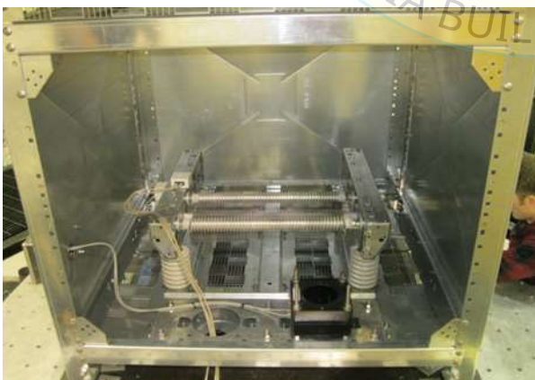
Side panel removed to photograph interior. Notice seismic bracing has been removed and number of insulators have been reduced.
