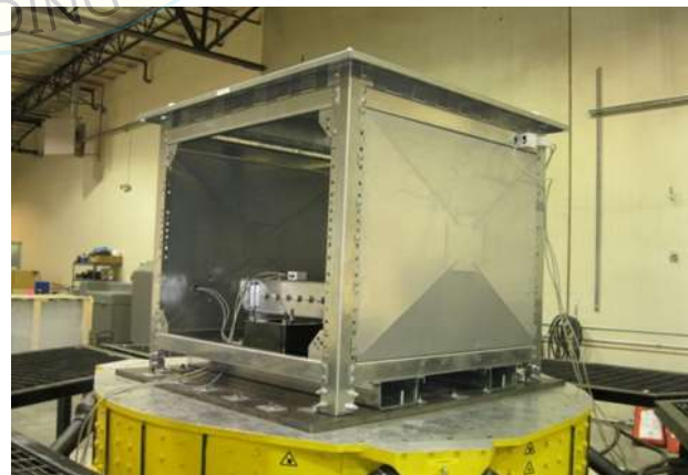
Unit mounted on shake table and ready for test (side panel removed for photograph).
