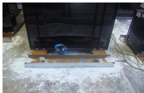
UUT4 Mounted to the Test Fixture by means of (8) ASTM A325 Bolts 3/4" Diameter
