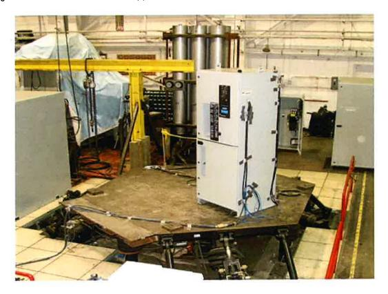
UUT maintained structural integrity and functionality as confirmed in post test inspection and operation checks. UUT was full of contents.
