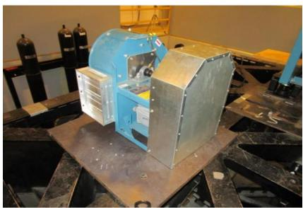
Rigidly Mounted to table. Fan bolted to table with (6) 3/8" dia. A307 bolts.
