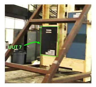
Rigid wall mounted - recessed using four (4) 1.25" long deck screws into the wood wall framing. Unit maintained structural integrity and remained functional per manufacturer requirement after shake table test. Contents were included in testing per operating conditions.
