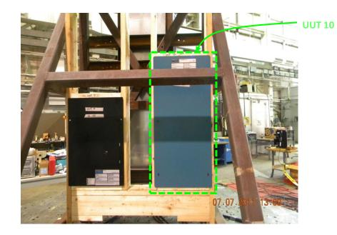
Rigid wall mounted - recessed using four (4) 1.25"-long deck screws: one (1) screw at each corner. Unit maintained structural integrity and remained functional per manufacturer requirement after shake table test. Contents were included in testing per operating conditions.
