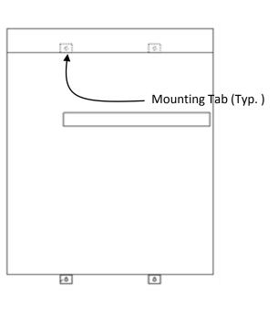
Rigid wall mounted using four (4) 5/16" hex head screws.
