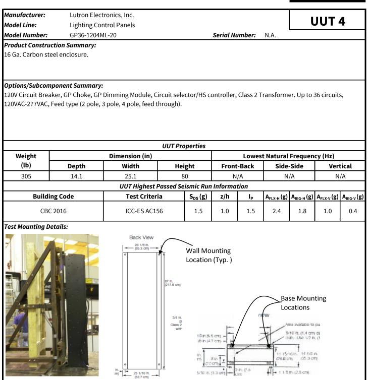
Rigid wall and floor mounted using six (6) 1/2" Grade 5 bolts: four (4) to the wall fixture, and two (2) into the shake table platen along the front of the unit.
