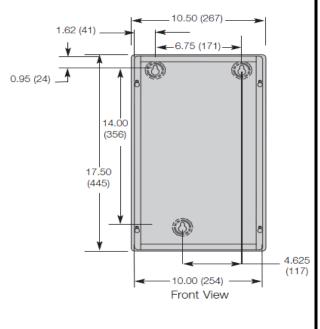
Rigid wall mounted - recessed using three (3) 5/16"Grade 5 bolts at the locations as shown in the above layout. Unit maintained structural integrity and remained functional per manufacturer requirement after shake table test. Contents were included in testing per operating conditions.
