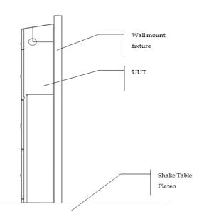
Rigid wall and base mounted with eight (8) 1/2" Grade 5 bolts: four (4) to the wall fixture, and four (4) into the table. Unit maintained structural integrity and remained functional per manufacturer requirement after shake table test. Contents were included in testing per operating conditions.
