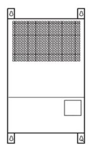
Rigid wall mounted using four (4) 5/16" hex head screws.
