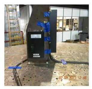
Rigid wall mounted - recessed using four (4) 5/16"Grade 5 bolts: one (1) at each corner. Unit maintained structural integrity and remained functional per manufacturer requirement after shake table test. Contents were included in testing per operating conditions.
