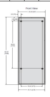
Rigid wall mounted with four (4) 5/16" Grade 5 bolts using the anchor layout as shown above. Unit maintained structural integrity and remained functional per manufacturer requirement after shake table test. Contents were included in testing per operating conditions.
