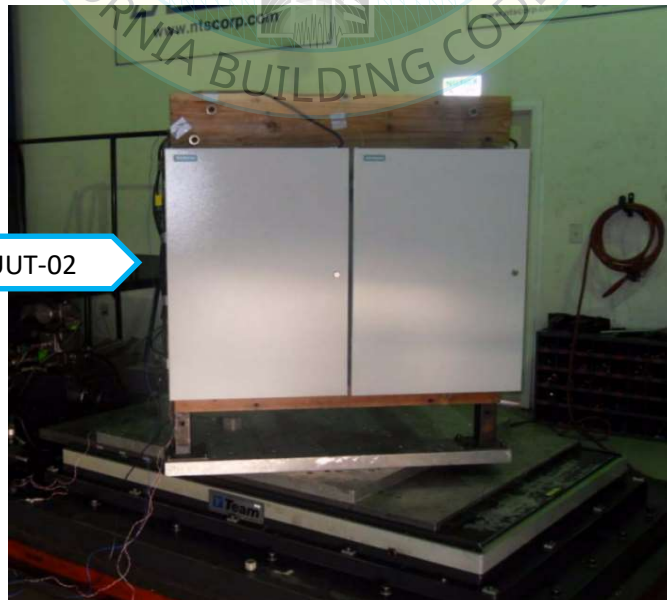
Overall view of UUT-02
