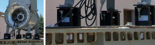
The unit was anchored to the table using four VMC MS-1C-150 spring isolators which were welded to the table surface.
