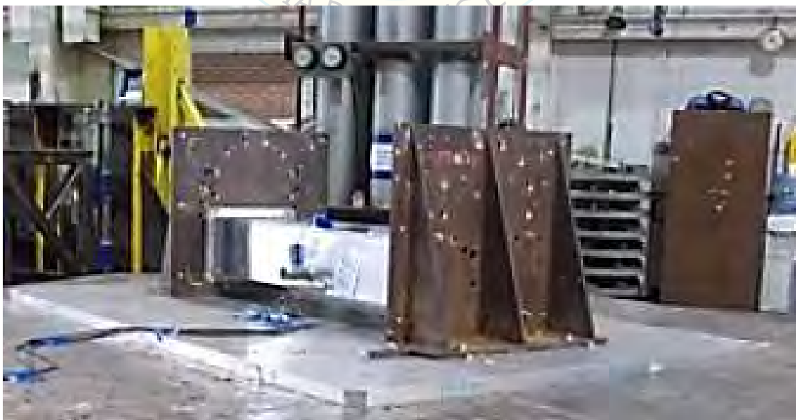
All units were filled with contents and maintained structural integrity and functionality after AC-156 test.
