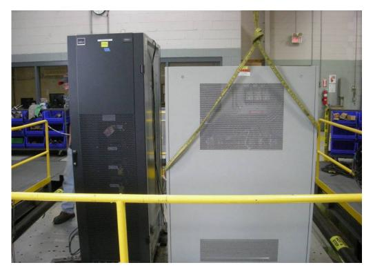
Figure 1: NX Bypass Distribution Cabinet (left) and PPC 200kVA UPS (right) Attachment Method: hard-mount - 5/8"dia bolts to table, angle brackets by Liebert
