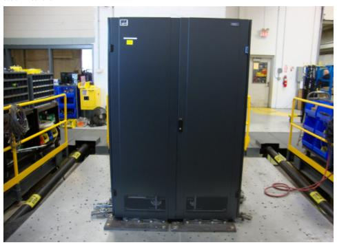
Figure 4: NX Wide Battery Cabinet Attachment Method: hard-mount - 5/8"dia bolts to table, angle brackets by Liebert
