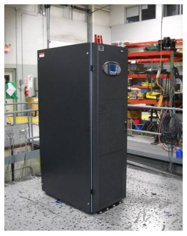
Figure 3: NX 40kVA UPS Attachment Method: hard-mount - 1/2"dia bolts to table, angle brackets by Liebert
