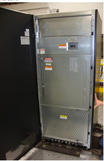
Figure 5: NX Narrow Battery Cabinet (front door open) Attachment Method: hard-mount - 5/8"dia bolts to table, angle brackets by Liebert
