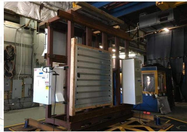
Mounting: Wall mounted flexible. Wall mounted using (34) 1/4-in sheet metal screws (6-in o.c., all four sides). Test fixture was base mounted spring vibration isolated using (4) Mason SSLFHC 1750 spring isolators.
