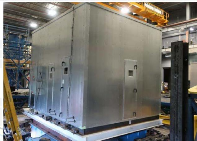
Mounting: Base mounted rigid using (12) 5/8-in diameter Grade 8 bolts. Each side wall (parallel to airflow) has (6) 6-in long L3x3x3/8-in brackets spaced 24-in o.c. Each bracket connects to the unit base with (2) 3/4-in diameter Grade 5 bolts.
