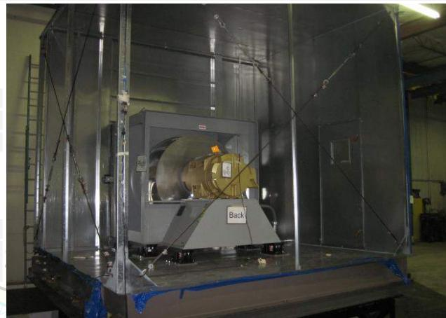
Mounting: Base mounted rigid using (16) 5/8-in diameter Grade 8 bolts. Each side wall (parallel to airflow) has (4) 6-in long L3x3x3/8-in brackets. Each bracket connects to the unit base with (2) 3/4-in diameter Grade 5 bolts.
