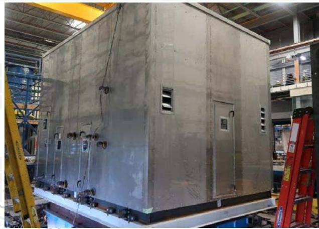
Mounting: Base mounted rigid using (16) 5/8-in diameter Grade 8 bolts. Each side wall (parallel to airflow) has (8) 6-in long L3x3x3/8-in brackets spaced 24-in o.c. Each bracket connects to the unit base with (2) 3/4-in diameter Grade 5 bolts.
