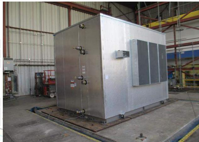
Mounting: Base mounted rigid using (12) 5/8-in diameter Grade 8 bolts and (10) 3-in long 5/16-in fillet welds. Each side wall (parallel to airflow) has (5) welds and (6) 6-in long L3x3x3/8-in brackets spaced 24-in o.c. Each bracket connects to the unit base with (2) 3/4-in diameter Grade 5 bolts.
