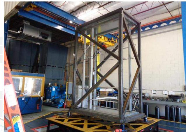
Mounting: Base/wall mounted flexible. Base/wall mounted to 16GA thick carbon steel panels using (28) 1/4-in carbon steel sheet metal screws (7 each flange of bulkhead on top and bottom, 14-in o.c. spacing, starting 2-in from end of bulkhead). Test fixture was base mounted spring vibration isolated using (4) Mason SSLFHB 1000 spring isolators.
