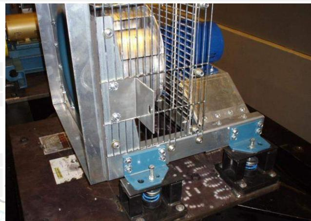
Mounting: Base mounted spring vibration isolated using (4) VMC MSS-1C-50 spring isolators using (4) 3/8-in diameter ASTM A307 bolts per isolator.
