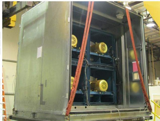
Mounting: Base mounted rigid using (28) 1/2-in diameter Grade 5 bolts spaced at 16-in o.c. around the perimeter.
