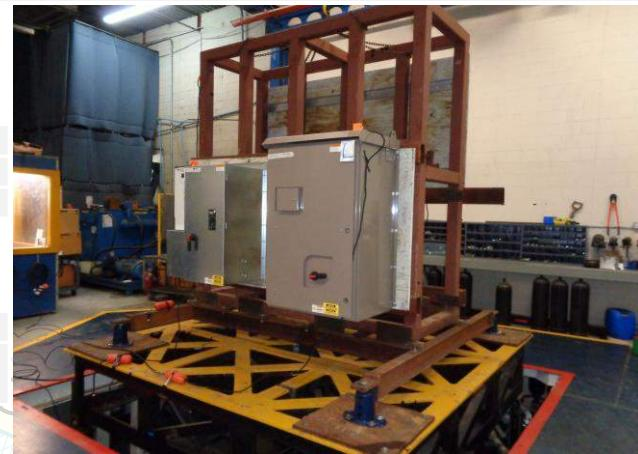
Mounting: Wall mounted flexible. Wall mounted using (10) 3/8-in diameter Grade 5 bolts. Test fixture was base mounted spring vibration isolated using (4) Mason SSLFHC 1750 spring isolators.
