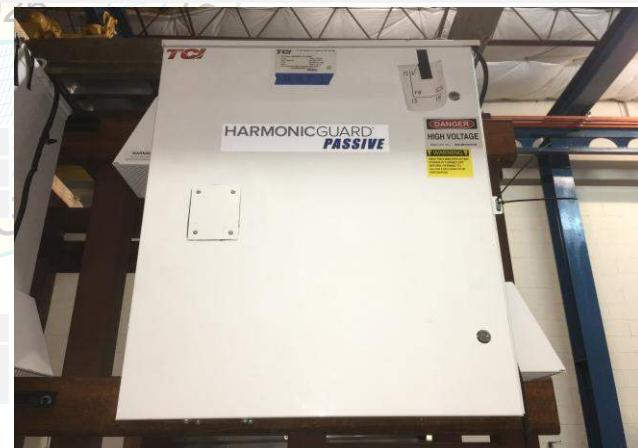
Importance Factor, I<sub>P</sub> = 1.5: Unit was full of operating content during the shake table test. Unit maintained structural integrity and remained functional per manufacturer requirement after shake table test.
