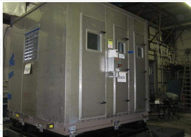
Mounting: Base mounted curb non-isolated on 14-in tall VMC P6000S curb using (6) 4in long 3/8-in fillet welds. Each side wall (parallel to airflow) has (3) welds spaced 44-in o.c. Curb was base mounted rigid using (20) 5/8-in diameter Grade 8 bolts evenly spaced around perimeter in groups of (2).
