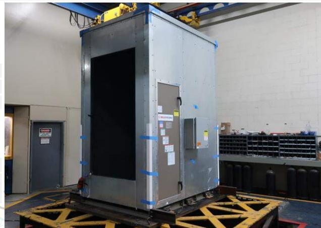
Mounting: Base mounted rigid using (6) 3/4-in diameter Grade 5 bolts. Each side wall (parallel to airflow) has (3) 6-in long L3x3x3/8-in brackets spaced 24-in o.c. Each bracket connects to the unit base with (2) 3/4-in diameter Grade 5 bolts.
