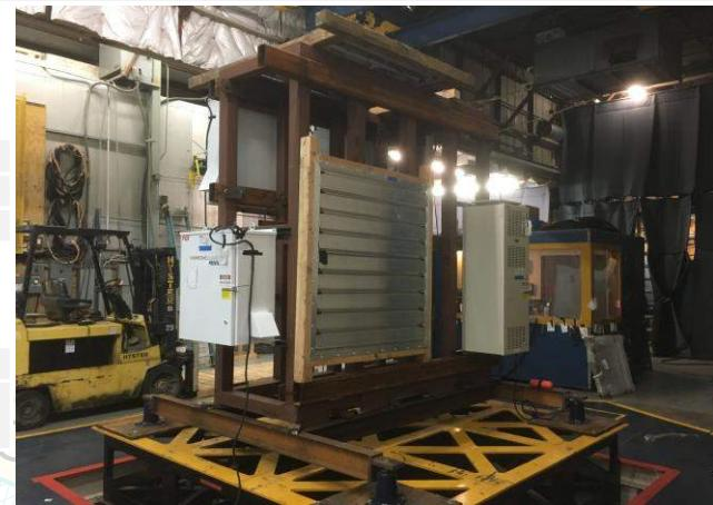
Mounting: Horizontal surface mounted flexible. Horizontal surface mounted using (34) 1/4-in sheet metal screws (6-in o.c., all four sides). Test fixture was base mounted spring vibration isolated using (4) Mason SSLFHC 1750 spring isolators.
