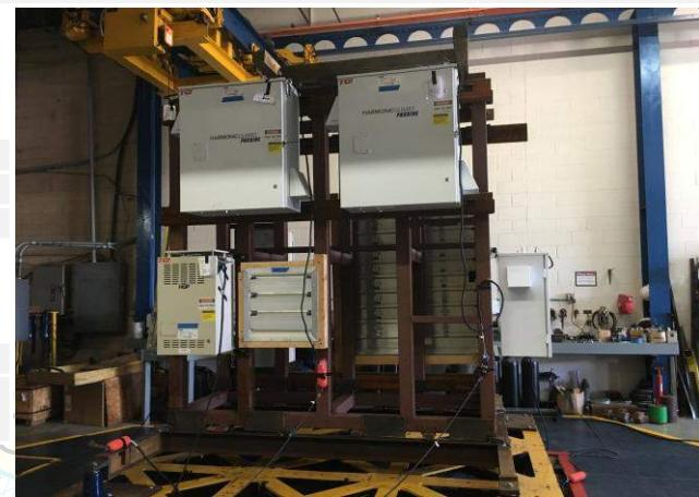
Mounting: Wall mounted flexible. Wall mounted using (16) 1/4-in sheet metal screws (6-in o.c., all four sides). Test fixture was base mounted spring vibration isolated using (4) Mason SSLFHC 1750 spring isolators.
