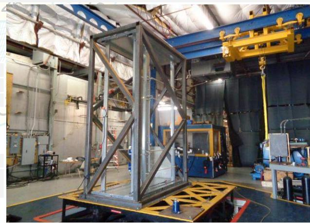
Mounting: Base/wall mounted rigid. Mounting was identical to above except test fixture was base mounted rigid.
