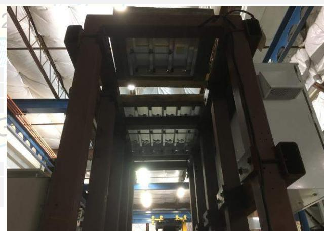
Mounting: Horizontal surface mounted rigid. Mounting was identical to above except test fixture was base mounted rigid.
