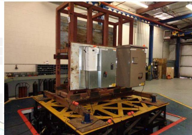
Mounting: Wall mounted flexible. Wall mounted using (4) 3/8-in diameter Grade 5 bolts. Test fixture was base mounted spring vibration isolated using (4) Mason SSLFHC 1750 spring isolators.
