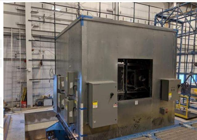
Mounting: Base mounted rigid using (28) 12-in long 3/8-in fillet welds. Welds are evenly spaced at 24-in o.c. around the full perimeter.
