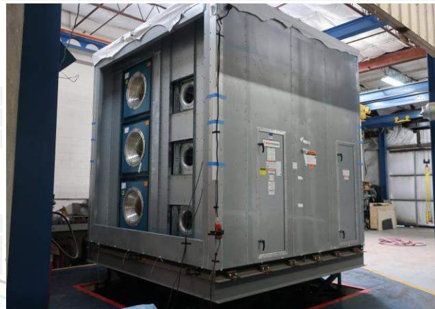
Mounting: Base mounted rigid using (12) 3/4-in diameter Grade 5 bolts. Each side wall (parallel to airflow) has (6) 6-in long L3x3x3/8-in brackets spaced 24-in o.c. Each bracket connects to the unit base with (2) 3/4-in diameter Grade 5 bolts.
