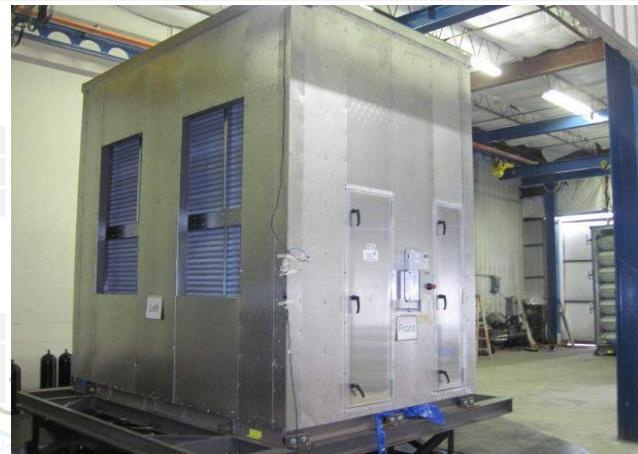
Mounting: Base mounted rigid using (12) 5/8-in diameter Grade 8 bolts. Each side wall (parallel to airflow) has (3) 6-in long L3x3x3/8-in brackets. Each bracket connects to the unit base with (2) 3/4-in diameter Grade 5 bolts.
