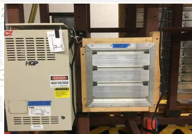
Mounting: Wall mounted rigid. Mounting was identical to above except test fixture was base mounted rigid.
