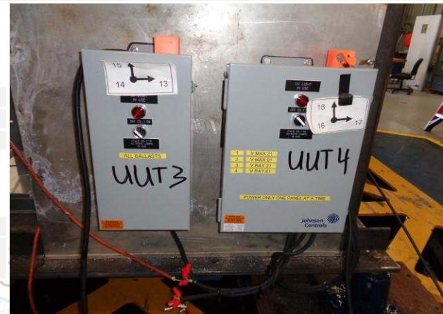
Mounting: Wall mounted flexible. Wall mounted to 16GA thick carbon steel panel using (4) 3/8-in diameter Grade 2 bolts into standard rivet nuts. Test fixture was base mounted spring vibration isolated using (4) Mason SSLFHB 1000 spring isolators.
