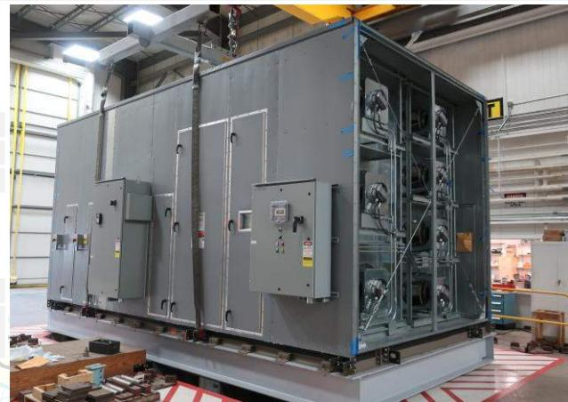
Mounting: Base mounted rigid using (24) 3/4-in diameter Grade 8 bolts. Each side wall (parallel to airflow) has (12) 6-in long L3x3x3/8-in brackets spaced 24-in o.c. Each bracket connects to the unit base with (2) 3/4-in diameter Grade 5 bolts.
