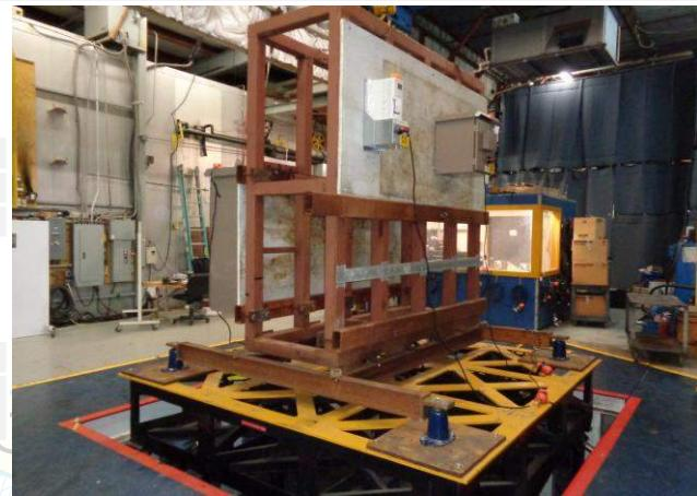
Mounting: Wall mounted flexible. Wall mounted using (4) 3/8-in diameter lag bolts. Test fixture was base mounted spring vibration isolated using (4) Mason SSLFHC 1750 spring isolators.
