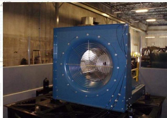
Mounting: Base mounted spring vibration isolated using (2) VMC MSSH-1E-530N and (2) MSSH-1E-825N spring isolators using (4) 5/8-in diameter ASTM A325 bolts per isolator.
