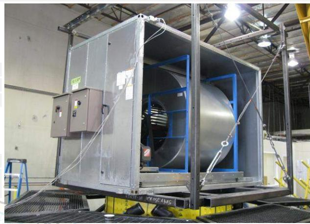
Mounting: Base mounted rigid using (8) 3/8-in diameter Grade 5 bolts. Each end wall (perpendicular to airflow) has (2) brackets located near the corners.
