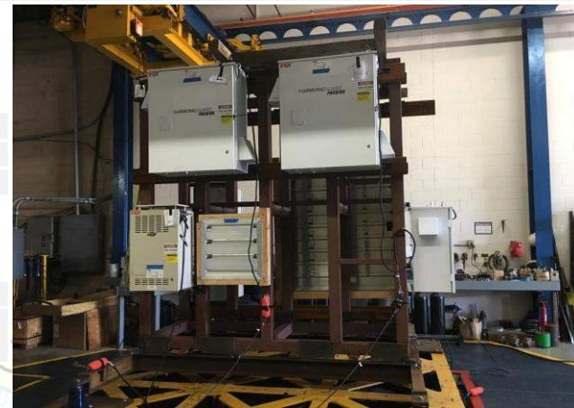
Mounting: Wall mounted flexible. Wall mounted to P1000 Unistrut rails using (4) 3/8-in diameter Grade 2 bolts to P1008 Unistrut channel nuts. Unistrut rails mounted to test fixture using (2) 3/8-in diameter Grade 8 bolts per rail (2 rails, 4 bolts total). Test fixture was base mounted spring vibration isolated using (4) Mason SSLFHC 1750 spring isolators.
