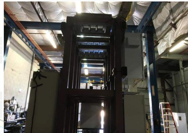
Mounting: Horizontal surface mounted flexible. Horizontal surface mounted using (16) 1/4-in sheet metal screws (6-in o.c., all four sides). Test fixture was base mounted spring vibration isolated using (4) Mason SSLFHC 1750 spring isolators.
