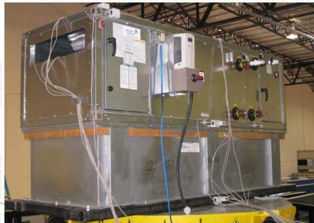
Mounting: Base mounted curb non-isolated on 24-in tall 14GA MicroMetl curb using #12 sheet metal screws spaced at 7.5-in o.c. around the perimeter. Curb was base mounted rigid using 1/2-in diameter bolts spaced at 18-in o.c. around the perimeter.
