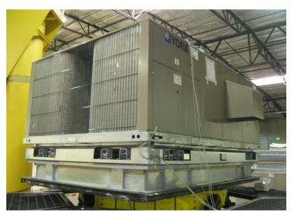
UUT3b was tested on a spring-isolated roof curb by ProVent. The curb had ten 10-gage anchoring pockets, four on each long side of the curb and one on each short side. The unit was attached to each of the pockets using five #14x1-1/2-inch TEK screws. The curb was attached to the 3/4-inch thick steel shake table interface plate with twelve 1/2-inch diameter Grade 5 bolts, four on each long side of the curb and two on each short side. The bolts were evenly spaced.
