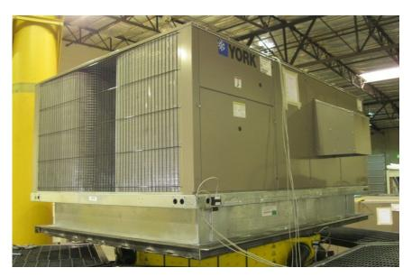
UUT3a was tested on a rigid roof curb by MicroMetl. The curb had eight 10-gage anchoring pockets, four on each long side of the curb. The unit was attached to each of the pockets using ten #12x1/2-inch TEK screws. The curb was attached to the 3/4-inch thick steel shake table interface plate with sixteen 3/8-inch diameter Grade 5 bolts, six on each long side of the curb and four on each short side, with each side sharing a bolt on the corners. The bolts were evenly spaced.
