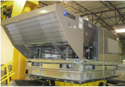
UUT2b was tested on a spring-isolated roof curb by ProVent. The curb had ten 10-gage anchoring pockets, four on each long side of the curb and one on each short side. The unit was attached to each of the pockets using five #14x1-1/2-inch TEK screws. The curb was attached to the 3/4-inch thick steel shake table interface plate with twelve 1/2-inch diameter Grade 5 bolts, four on each long side of the curb and two on each short side. The bolts were evenly spaced.
