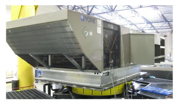
UUT1a was tested on a rigid roof curb by Ruskin. The curb had twelve 1/8-inch thick anchoring pockets, four on each side of the long direction of the curb and two on each short side. The unit was attached to each of the pockets using two 1/4-20 x 5-inch self-drilling screws. The curb was attached to the 3/4-inch thick steel shake table interface plate with ten 1/2-inch diameter Grade 5 bolts, one-foot in from each corner and one centered on each of the long sides.
