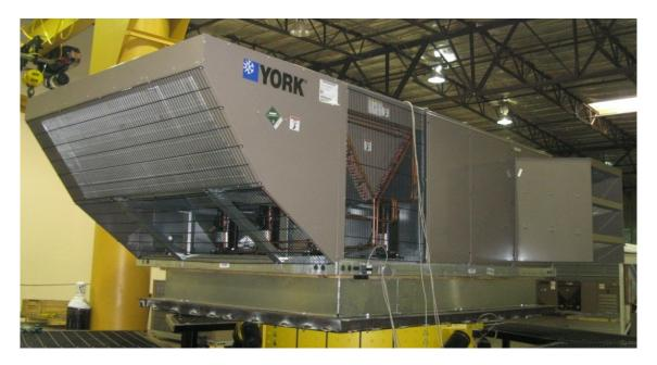
UUT5a was tested on a rigid roof curb by Ruskin. The curb had twelve 1/8-inch thick anchoring pockets, four on each side of the long direction of the curb and two on each short side. The unit was attached to each of the pockets using two 1/4-20 x 5-inch self-drilling screws. The curb was attached to the 3/4-inch thick steel shake table interface plate with ten 1/2-inch diameter Grade 5 bolts, one-foot in from each corner and one centered on each of the long sides.
