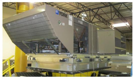
UUT1b was tested on a spring-isolated roof curb by MicroMetl. The curb had eight 10-gage anchoring pockets, four on each long side of the curb. The unit was attached to each of the pockets using seven #12x1/2-inch TEK screws. The curb was attached to the 3/4-inch thick steel shake table interface plate with twelve 1/2-inch diameter Grade 5 bolts, four on each long side of the curb and two on each short side.
