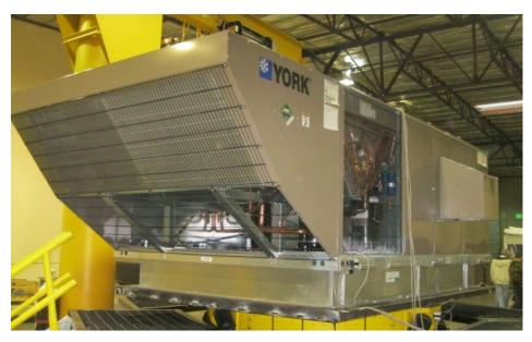
UUT4a was tested on a rigid roof curb by MicroMetl. The curb had eight 10-gage anchoring pockets, four on each long side of the curb. The unit was attached to each of the pockets using ten #12x1/2-inch TEK screws. The curb was attached to the 3/4-inch thick steel shake table interface plate with sixteen 3/8-inch diameter Grade 5 bolts, six on each long side of the curb and four on each short side, with each side sharing a bolt on the corners. The bolts were evenly spaced.
