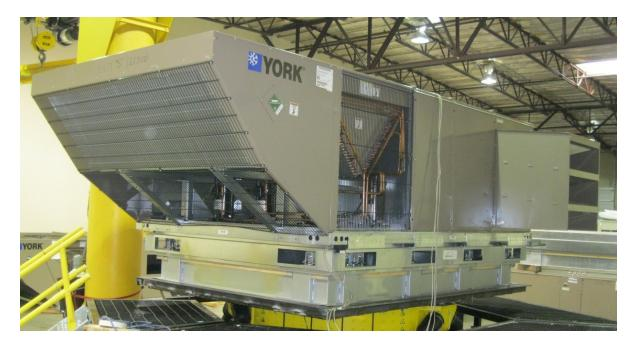
UUT5b was tested on a spring-isolated roof curb by MicroMetl. The curb had eight 10-gage anchoring pockets, four on each long side of the curb. The unit was attached to each of the pockets using seven #12x1/2-inch TEK screws. The curb was attached to the 3/4-inch thick steel shake table interface plate with twelve 1/2-inch diameter Grade 5 bolts, four on each long side of the curb and two on each short side.
