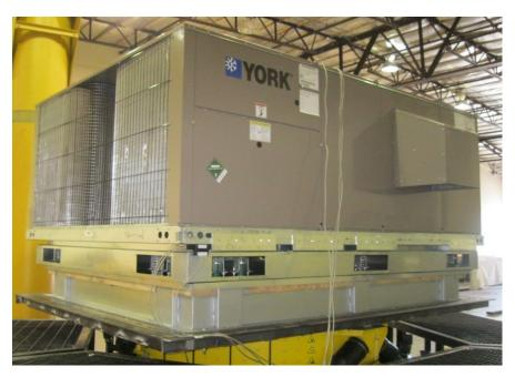
UUT6b was tested on a spring-isolated roof curb by MicroMetl. The curb had eight 10-gage anchoring pockets, four on each long side of the curb. The unit was attached to each of the pockets using seven #12x1/2-inch TEK screws. The curb was attached to the 3/4-inch thick steel shake table interface plate with twelve 1/2-inch diameter Grade 5 bolts, four on each long side of the curb and two on each short side.
