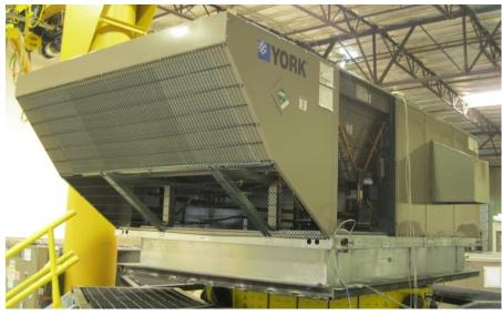
UUT2a was tested on a rigid roof curb by MicroMetl. The curb had eight 10-gage anchoring pockets, four on each long side of the curb. The unit was attached to each of the pockets using ten #12x1/2-inch TEK screws. The curb was attached to the 3/4-inch thick steel shake table interface plate with sixteen 3/8-inch diameter Grade 5 bolts, six on each long side of the curb and four on each short side, with each side sharing a bolt on the corners. The bolts were evenly spaced.
