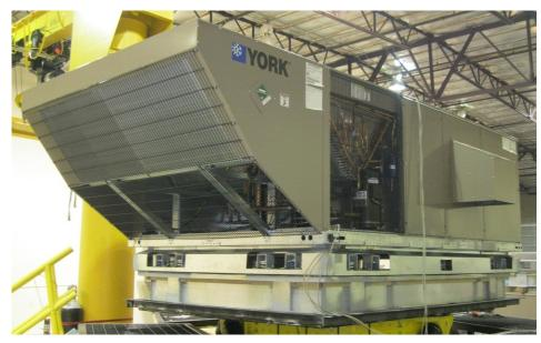
UUT4b was tested on a spring-isolated roof curb by ProVent. The curb had ten 10-gage anchoring pockets, four on each long side of the curb and one on each short side. The unit was attached to each of the pockets using five #14x1-1/2-inch TEK screws. The curb was attached to the 3/4-inch thick steel shake table interface plate with twelve 1/2-inch diameter Grade 5 bolts, four on each long side of the curb and two on each short side. The bolts were evenly spaced.
