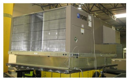
UUT6a was tested on a rigid roof curb by Ruskin. The curb had twelve 1/8-inch thick anchoring pockets, four on each side of the long direction of the curb and two on each short side. The unit was attached to each of the pockets using two 1/4-20 x 5-inch self-drilling screws. The curb was attached to the 3/4-inch thick steel shake table interface plate with ten 1/2-inch diameter Grade 5 bolts, one-foot in from each corner and one centered on each of the long sides.
