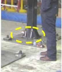
CEM rigid base mounted to frame with (16) 3/4" A490 bolts. Frame rigid mounted to fixture plates with (16) 7/8" A490 bolts. Unit maintained structural integrity and remained functional per manufacturer requirement after shake table test. Contents were included in testing per operating conditions.
