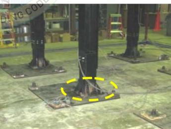
CEM rigid base mounted to frame with (16) 3/4" A490 bolts. Frame rigid mounted to fixture plates with (16) 7/8" A490 bolts. Unit maintained structural integrity and remained functional per manufacturer requirement after shake table test. Contents were included in testing per operating conditions.
