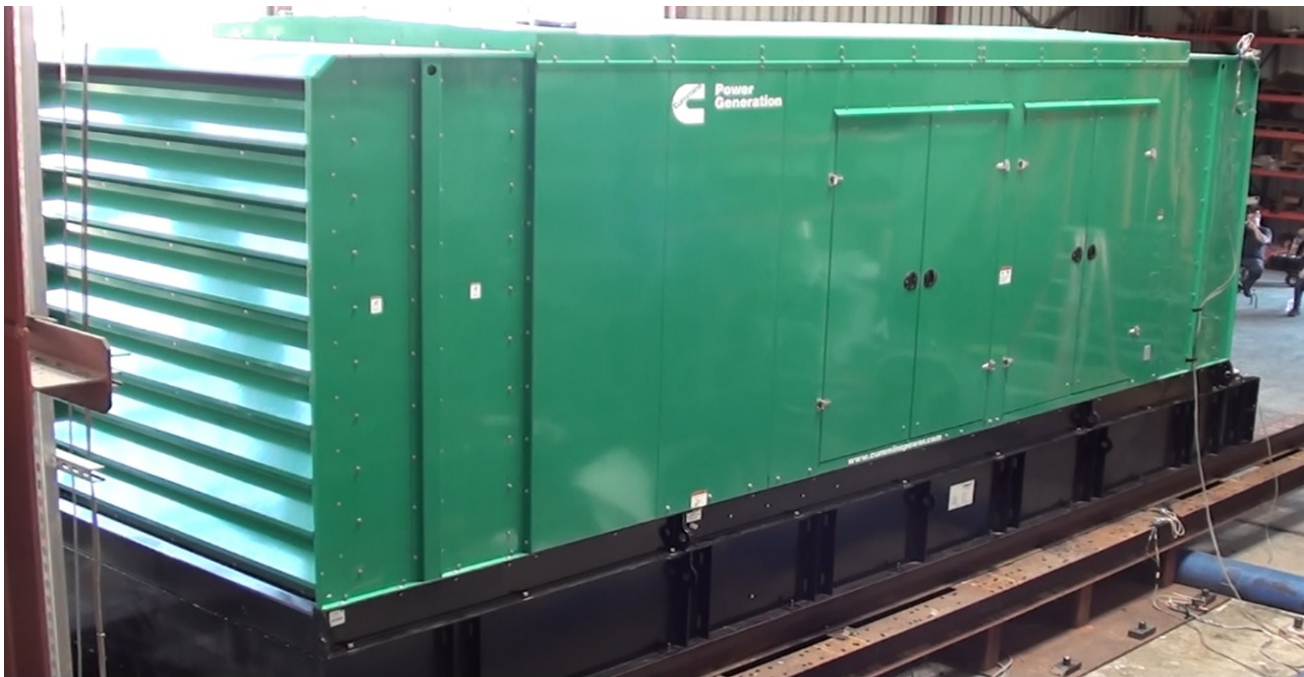
Equipment layout on table. Genset secured to enclosure base via (10) VMC M2SSH-1E-3400N spring isolators. Subbase tank secured to fixture using (18) 3/4" dia SAE Grade 8 bolts.
