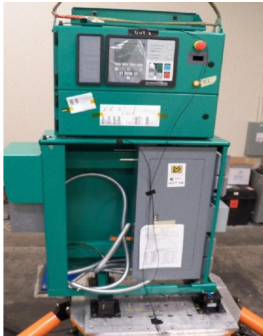
Equipment layout on table. Support assembly secured to fixture using (4) M10x1.5x25 Class 8.8 bolts, torqued 47-57 Nm.
