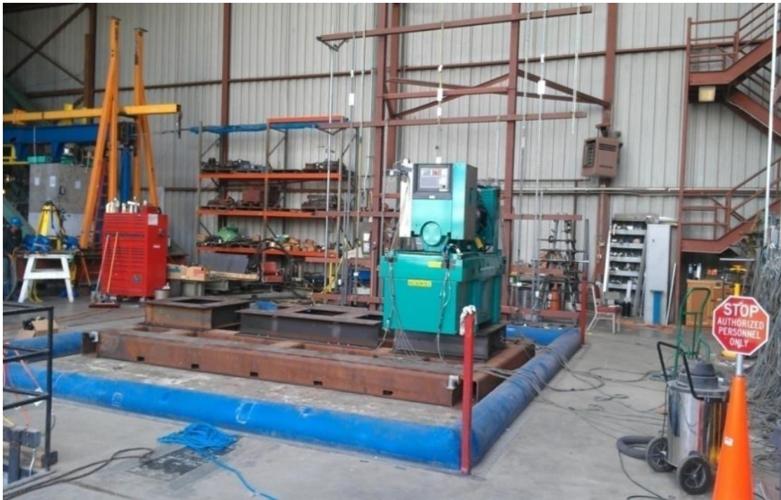
Equipment layout on table. Sub-base tank secured to fixture using (4) 3/4" dia ASTM 325 bolts.
