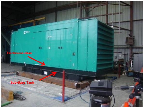
Equipment layout on table. Sub-base tank secured to fixture using (12) 3/4" dia SAE Grade 8 bolts.
