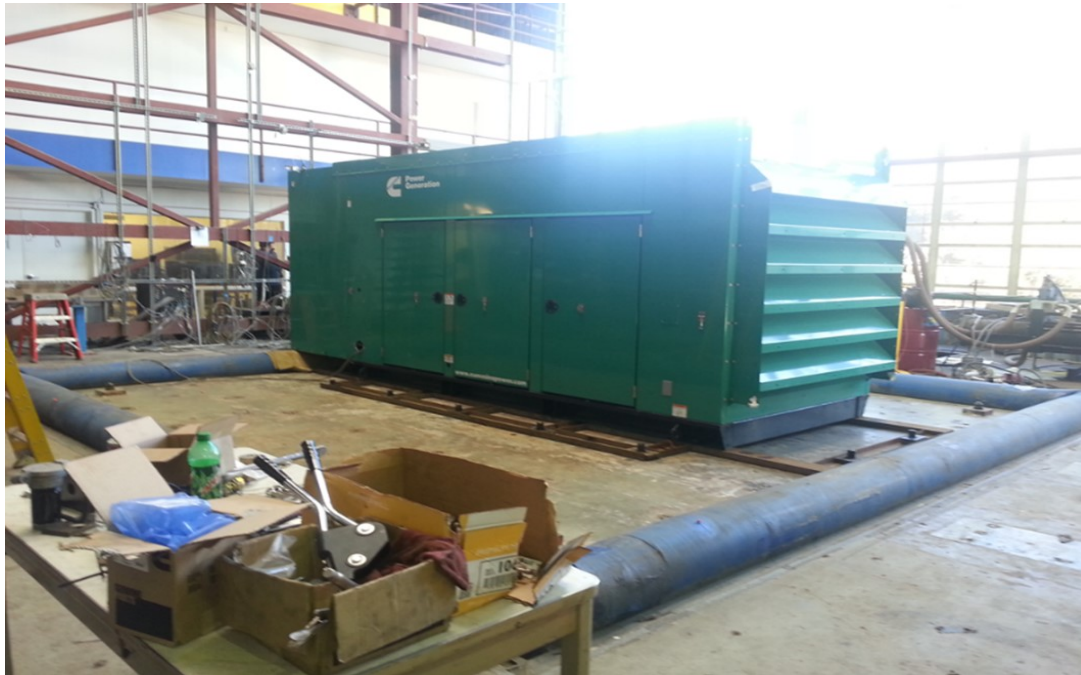
Equipment layout on table. Genset secured to enclosure base via (4) EBCO 4990-60 duro elastomer isolators. Enclosure base secured to the fixture using (4) 3/4" dia ASTM 325 bolts.
