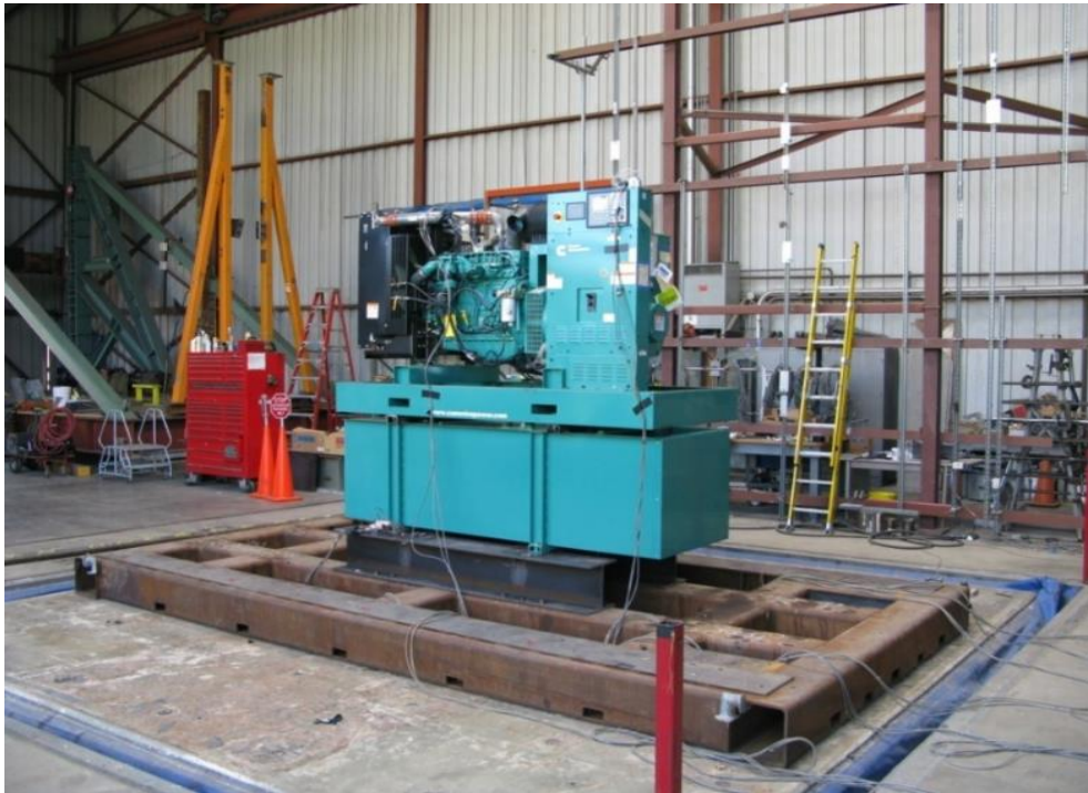
Equipment layout on table. Sub-base tank secured to fixture using (4) 3/4" dia ASTM 325 bolts.
