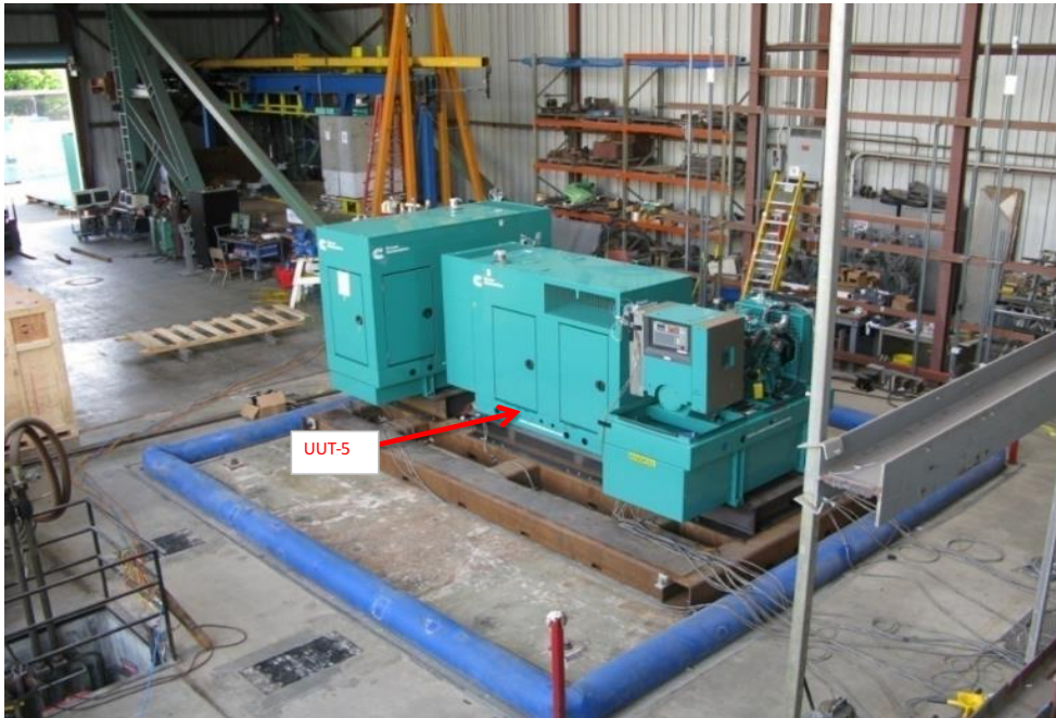
Equipment layout on table. Genset secured to fixture using (4) 3/4" dia ASTM 325 bolts.
