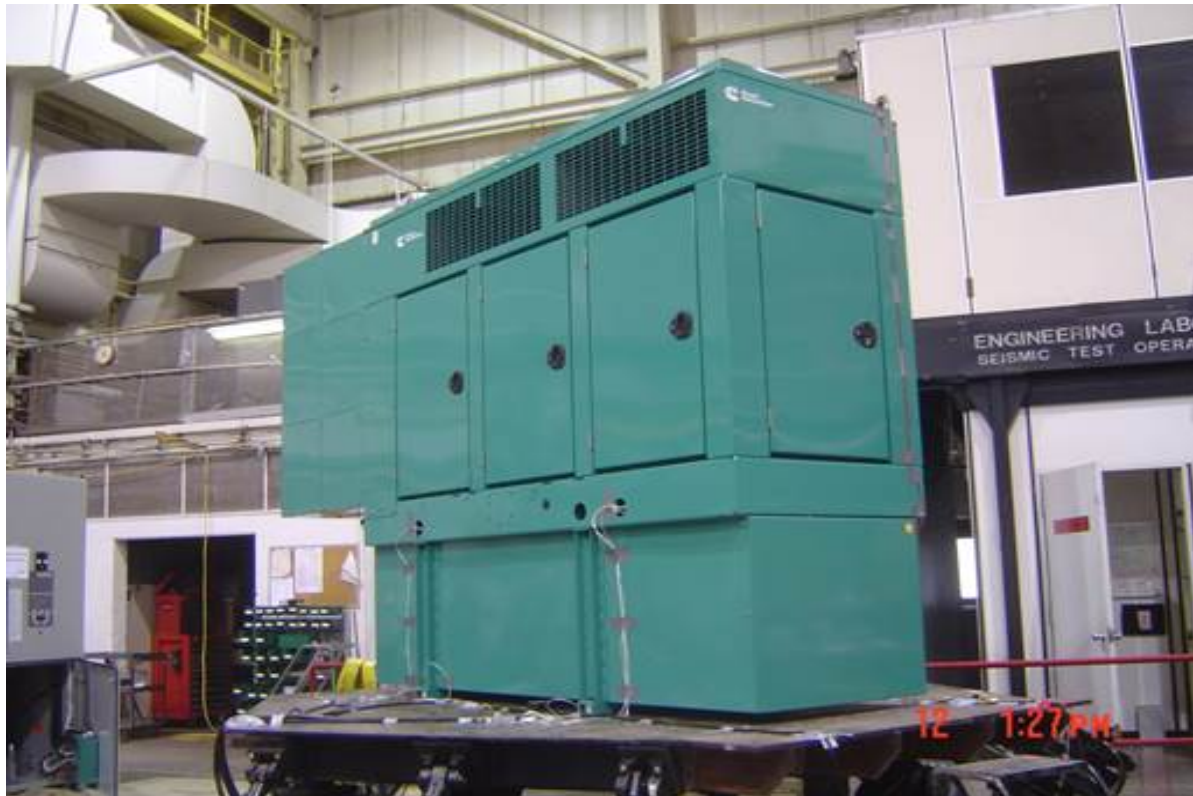
Equipment layout on table. Subbase tank secured to fixture using (2) 3/4" dia SAE grade 5 bolts and (2) 3/4" SAE grade 9 strain measurement bolts.
