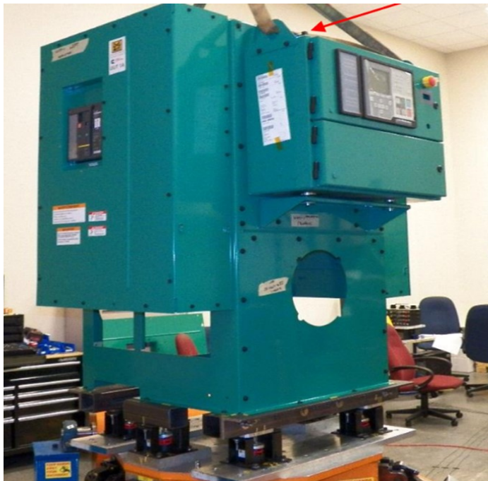
Equipment layout on table. Support assembly secured to fixture using (4) VMC MSS-1C-150 spring isolators.
