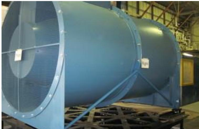
The 730 QSL fan with VMC isolators was mounted to the ANCO shake table as specified in the installation instructions. The fan was then mounted to the (4) VMC isolators. The isolators were attached to 1 inch adapter plates and mounted to the shake table. The isolator's air gap was set to 1/4" before the test. Component was full of content during test and maintained structural integrity and functionality after the shake test.
