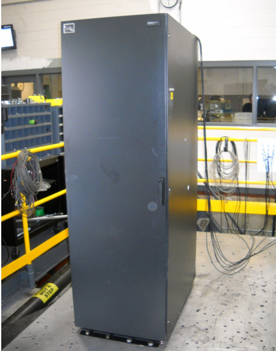
Figure 2: UUT-10 45kVA BDC Attachment Method: hard-mount - 1/2" dia bolts to table, angle brackets by Liebert
