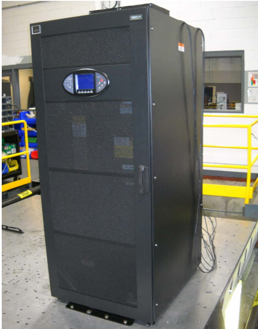
Figure 4: UUT-9 90kVA UPS Attachment Method: hard-mount - 1/2" dia bolts to table, angle brackets by Liebert
