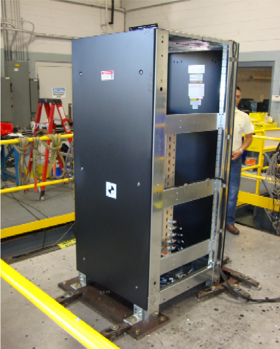
Figure 7: UUT-2 Wide Junction Cabinet (tested without left and right side panels) Attachment Method: hard-mount - (4)-3/4"dia bolts to table, angle brackets by Liebert
