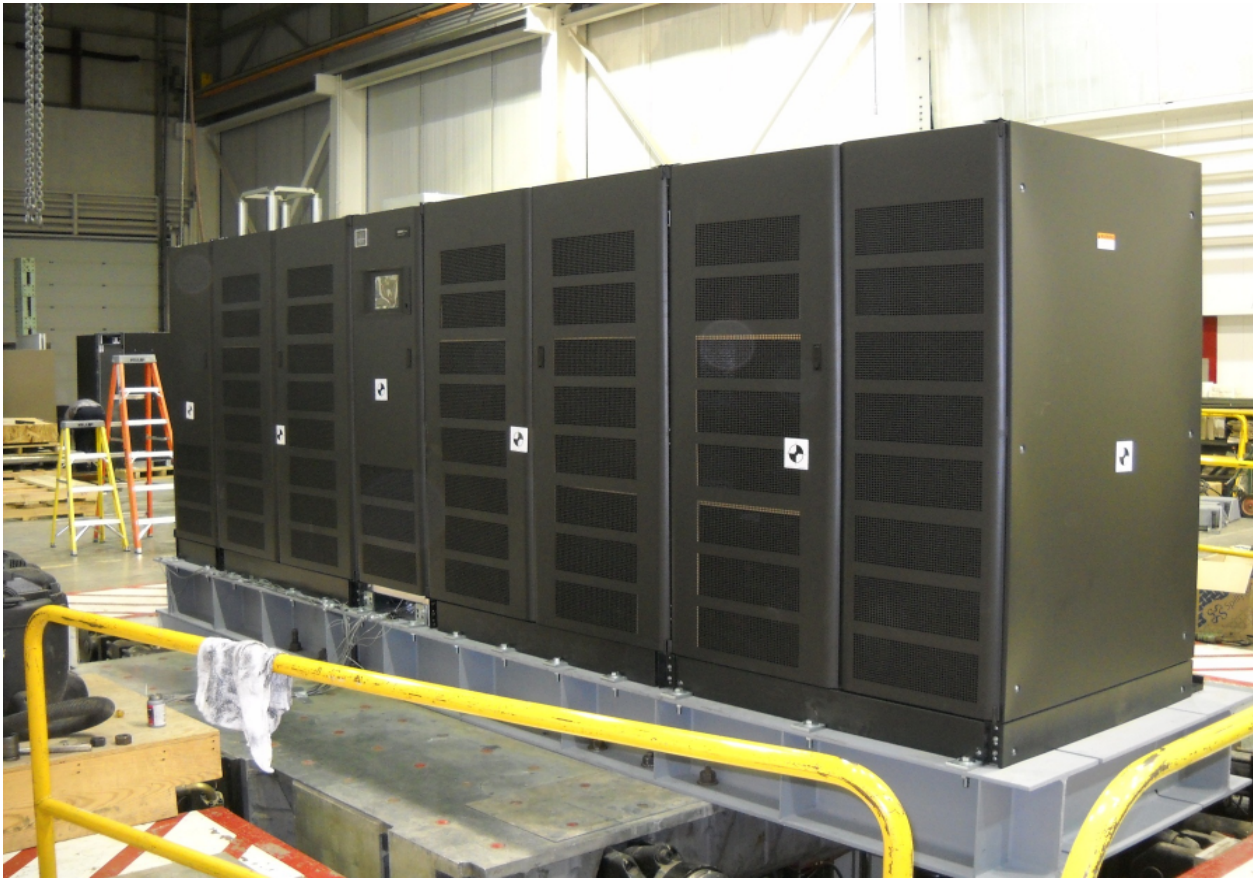
Figure 3: UUT-4 1100kVA UPS Attachment Method: hard-mount - (30)-3/4"dia bolts to fixture, angle brackets by Liebert
